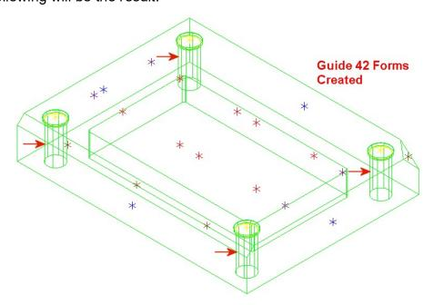
Taking a closer look at the drill form, you will notice that at the top of the smaller cylinder / through hole, a yellow arc is created. This represents the cylinder that will be reamed.
