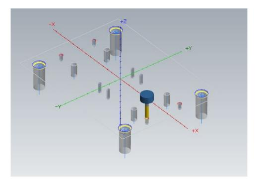
You have created drilling forms on a 2D drawing, processed the part and generated toolpaths for the same in a manner of minutes!
