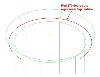
We will now create some forms on non-standard planes. Click on **Create Forms - Solids**, **B\_Flat\_Drill** and select the **Flat\_Drill\_12mm** form, right click and select **Drill Solid**.
