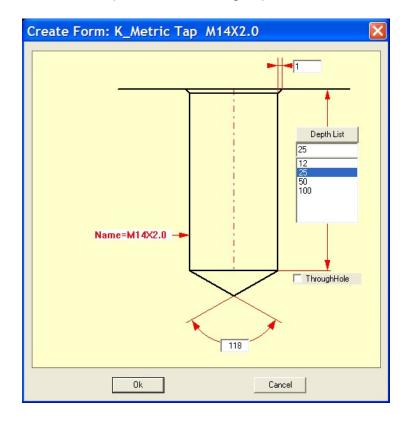
Set the parameters as shown above. Notice that we are creating a 1mm chamfer and creating it as a blind hole (**ThroughHole** unchecked). Click on OK
