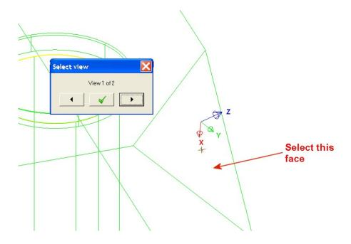
Once the new plane is set, select the brown point on the face as the **point** for drilling. Click on **Enter**.
