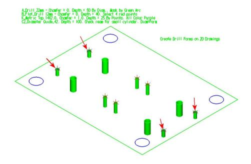
To indicate a Tap form, ProDrill also creates a 270 degree red arc on top of the cylinder to be tapped. Notice that the arc is created below the chamfer. The image on the right shows that the tap form ends in a tooltip (angle used in the Forms Parameters).
