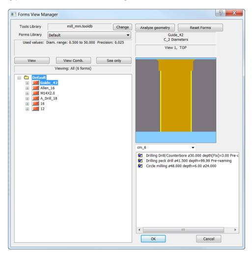
Notice that the holes that need to be tapped or reamed are all automatically recognized. At this point the toolpath can be generated for all the operations and you can backplot the toolpath or verify it to make sure it is exactly what you wanted.
