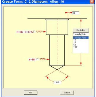
Change the settings as shown above. Disable the reaming of this drill form for the cylinders. Click on OK Click on the **8 red** points (Mastercam color 12). Click on **Enter**. The following will be the result.
