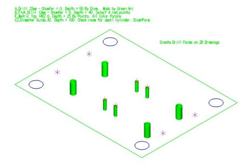
Click on **Create Forms - Surfaces**, select the tab for the **Tap** and click on **K\_Metric Tap**. Right click on the **M14X2.0** form and click on "**Create Surface Form**". The form creation parameters dialog is presented:
